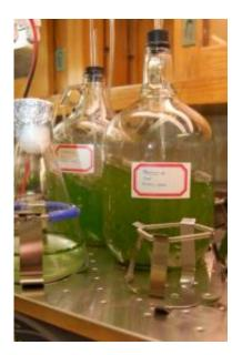
Researchers at the Ames Laboratory are growing several strains of algae to test nanofarming technology that uses sponge-like mesoporous nanoparticles to extract biofuel oils from the organisms. Credit: U.S. Dept. of Energy's Ames Laboratory
