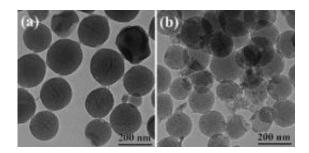
This micrograph shows the sponge-like mesoporous nanoparticles developed by researchers at Ames Laboratory to harvest biofuel oils from algae without harming the organisms. Credit: U.S. Dept. of Energy's Ames Laboratory
