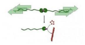
A catalyst can be switched from a dormant to an active state by pulling on a polymer chain, a "molecular ripcord". Credit: Rint Sijbesma
