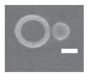
An image of the metallic ring and disk. The scale bar shows 200 nanometres.
