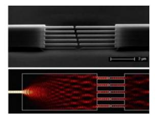
Electronmicroscopic image of array (top) and simulation of lightwaves through array (bottom). Credit: Li, Pernice, Tang
