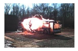
A mass transit bus is bombed in a test to see if prototype forensic cameras onboard will survive. Credit: DHS S&T
