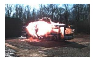
A mass transit bus is bombed in a test to see if prototype forensic cameras onboard will survive. Credit: DHS S&T
