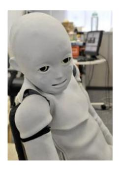
A "Child-robot with Biomimetic Body" or CB2, follows an object with his eyes at a laboratory in Osaka University
