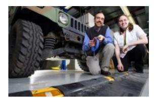
Douglas Adams, a Purdue associate professor of mechanical engineering, and graduate student Tiffany DiPetta are working to develop a technology that detects damage to critical suspension components in military vehicles simply by driving over a speed bumplike "diagnostic cleat" containing sensors. The researchers have tested the system in experiments with high-mobility multipurpose wheeled vehicles, or HMMWVs, commonly known as Humvees. Credit: Purdue News Service photo/Andrew Hancock
