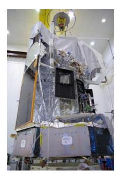
Herschel being weighed before fuelling. The measurements taken will serve as the baseline from which the final spacecraft mass will be derived after fuelling. The expected mass at launch is about 3400 Kg. Credits: ESA
