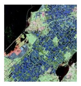
The colour composite of a RADARSAT-2 polarimetric radar image acquired over the Flevoland test site in the Netherlands on 4 April 2009. The different colours reflect the type and condition of the land cover. Field boundaries are clearly visible in this area, which is mostly agricultural. The dark areas correspond to water surrounding this area of reclaimed land, the very bright areas to urban settlements and the pink/blue area to middle-left is a nature reserve. Credits: MDA Geospatial Services
