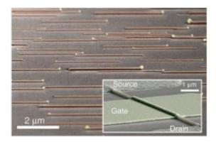
A scanning electron microscope image of self-assembled and self-aligned, planar gallium arsenide nanowires. The inset shows a field effect transistor fabricated with one of the nanowires.
