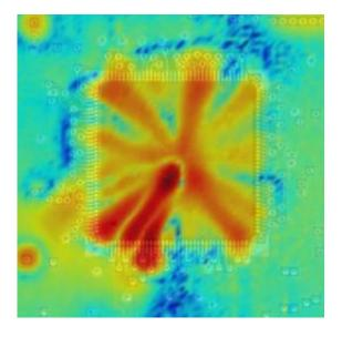
A near-field scanner can determine the electromagnetic field of any chip on the board. Credit: Fraunhofer ENAS
