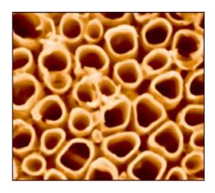
Scanning electron microscope image of typical titania nanotubes for a photocatalytic cell to produce hydrogen gas from water. Nanotubes average roughly 90-100 nanometers in diameter.
