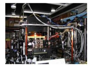
This is a strontium atomic clock operating at JILA, University of Colorado. Laser light is used to cool and manipulate the atoms for optimal operation of the clock. Carefully designed magnetic field coils compensate for the Earth magnetic field. Credit: University of Colorado
