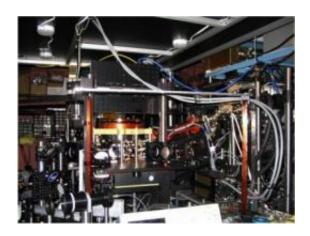
This is a strontium atomic clock operating at JILA, University of Colorado. Laser light is used to cool and manipulate the atoms for optimal operation of the clock. Carefully designed magnetic field coils compensate for the Earth magnetic field. Credit: University of Colorado
