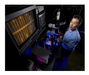
Sandia researcher Xinjian Zhou measures the electronic and optical properties of carbon nanotube devices in a probe station. The monitor shows the electrode layout on the device wafer; the nanotubes are positioned in the small horizontal gaps. Credit: (Photo by Randy Wong)
