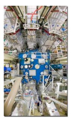
Composite photo shows all three floors containing the 264,000-pound, 10-meter diameter target chamber. Diagnostic instruments will be attached to the round hatches. Photo montage by Jacqueline McBride
