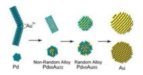
Schematic side view (top) and cross section (bottom) of as-made Pd, Pd68Au32, Pd45Au55, and Au nanomaterial during the galvanic replacement reaction.
