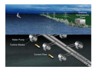
In the proposed hydrokinetic energy transfer system, the flow of water current causes turbine blades to rotate. The rotor's rotational speed is increased through a gearbox, which drives a high-pressure fluid pump. The high-pressure fluid would be transported though flexible tubes to a larger pipe and then to an efficient, onshore hydroelectric power plant.
