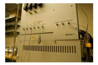
The Medusa gas chromatograph/mass spectrometer is used to analyze amounts of gases in air. Mühle used the device to track amounts of the fumigant sulfuryl fluoride in the atmosphere. Credit: Scripps Institution of Oceanography, UC San Diego
