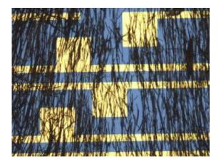
A view through the microscope shows microwires aligned in the same direction laying across electrodes below. Courtesy of Zhenan Bao
