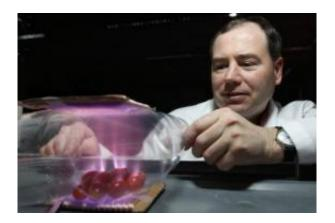
Kevin Keener's in-bag ozonation method creates ozone in packaged foods by using high-voltage coils to charge the gas inside sealed food packages, effectively killing any bacteria inside them. In this demonstration with a bag of tomatoes, helium has been added to a plastic bag because it glows, showing the ionization process. Credit: Purdue Agricultural Communication photo/Tom Campbell
