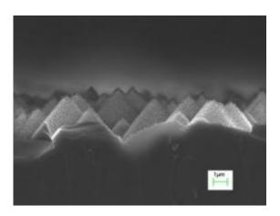
This image shows silicon pyramid structures etched for one minute using hydrogen fluoride/hydrogen peroxide/water solution. The resulting structure has roughness at the micro and nanometer scales. Credit: Image courtesy of C.P. Wong
