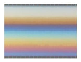
Overhead view of the NIST-Cornell 3-D nanofluidic device showing the different depth levels within the chamber as horizontal bands. The deepest, at the bottom, measures about 620 nanometers (slightly smaller than an average bacterium), while the shallowest, at the top, is about 60 nanometers (1,000 times smaller than the width of a human hair). The colors of the bands result from different mixing of white light components (interference) at each depth. Credit: NIST
