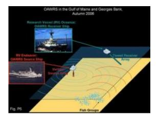
Schematic showing general setup of the imaging system used to study fish shoals. Graphic / Makris Lab, MIT; Ratilal Lab, NU
