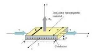
In this illustration of the system, salt water flows through a rectangular pipe under the influence of a perpendicular magnetic field, B0. The Lorentz force causes the charged sodium and chlorine ions to accumulate near the metal plates on the sides of the pipe, generating a constant electric field, E. Image credit: R. De Luca.
