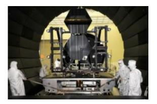
The Marshall Space Flight Center received two mirrors in the first shipment in December 2008. NASA and Ball Engineering technicians guide the mirrors into the center's X-ray and Cryogenic Facility's vacuum chamber for testing. Credit: NASA/MSFC, E. Given
