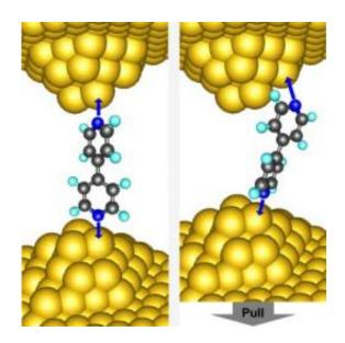
These schematics illustrate the "vertical" and "angled" molecular junction configurations for mechanically-induced switching. A study has revealed that electrical resistance through such a junction can be turned "on" and "off" simply by pushing (left) so that the configuration is vertical or and by pulling the junction so that the configuration is angled. Credit: The Molecular Foundry, Lawrence Berkeley National Laboratory
