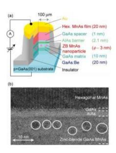
The top is a graphic representation of the overall device structure. The diameter is roughly that of a human hair. The bottom is a magnified image of the central part. The white spots are atoms and the white circles are the nano-magnets, the "working part" of the device. Credit: Pham Nam Hai
