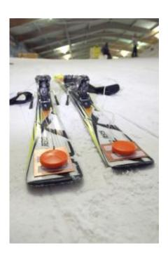
Small radio transmitters on skis provide information on whether the skis were parallel during a run for instance. © Dirk Mahler / Fraunhofer IFF
