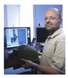
Akos Ledeczi holds a kevlar helmet with the microphones and network node attached that can turn the helmet into an accurate shooter location system. Credit: Steve Green, Vanderbilt University
