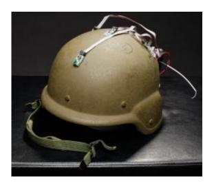
"Breadboard" version of the system mounted on a kevlar helmet. Image: Institute for Software Integrated Systems
