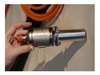
On Launch Pad 39A at NASA's Kennedy Space Center in Florida, a technician holds one of space shuttle Discovery's gaseous hydrogen flow control valves after its removal. Two of the three valves being removed will undergo detailed inspection. Photo Credit: NASA/Kim Shiflett
