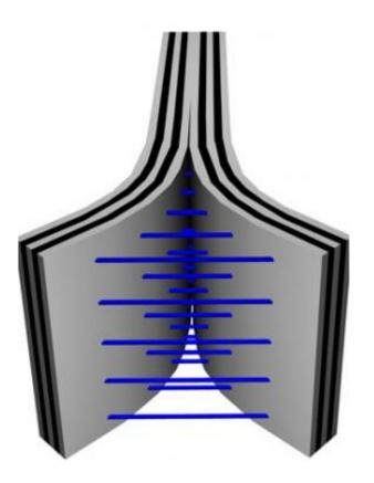
Schematic showing carbon nanotubes bridging the gap between plies of an advanced composite. Graphic courtesy / Wardle lab, MIT
