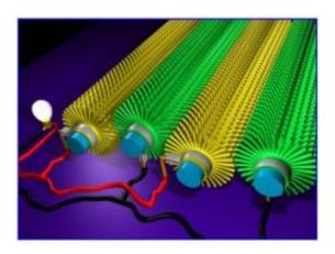
Pictured is a schematic illustration shows the microfiber-nanowire hybrid nanogenerator, which is the basis of using fabrics for generating electricity. Credit: Professor. Z. L. Wang and Dr. X. D. Wang, Georgia Institute of Technology.
