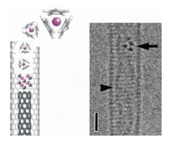
(Left) An illustration of the conversion of encapsulated cerium molecules to an inner nanotube. (Right) A transmission electron micrograph of a double-walled nanotube containing cerium (Ce@DWCNT). Arrows point to cerium ions (dark dots) and lines (inner tube). Scale bar is 1 nm. Credit: H. Shiozawa, et al. ©2009 The American Physical Society.
