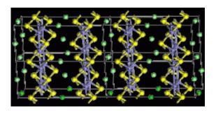
NIST research shows that magnetism plays a key role in iron pnictide superconductors' crystal structure. (Iron is purple; arsenic is yellow; calcium is green.) Only if the iron's magnetism is taken into account do calculations of the distance between these crystal layers match up with lab measurements. Magnetism's importance to their physical properties make it a likely factor in the iron pnictides' ability to superconduct, say team members. Credit: Yildirim, NIST
