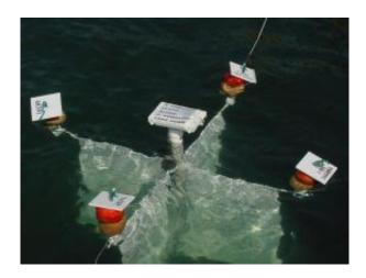
Close-up of drifter after deployment. Instructions are provided if the instrument washes ashore. (Credit: NOAA Fisheries)
