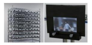
The live 3D TV system consists of (left) an array of 64 cameras that captures multi-view videos of a live scene and (right) an integral photography display with 60 viewing directions that reproduces an autostereoscopic 3D video of the scene. Image credit: Taguchi, et al. ©2008 IEEE.
