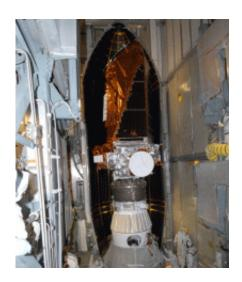
Workers attach the two-part payload fairing over the Kepler spacecraft in preparation for launch. The cover, designed to jettison shortly after launch, protects the spacecraft from the friction and turbulence as it speeds through the atmosphere during launch. Image credit: NASA/Jack Pfaller
