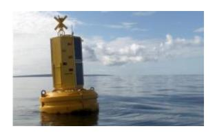
In this Sept. 4, 2008 photo provided by the Marine Institute of Ireland, a buoy that uses sensors in the ocean to collect data on water quality and sea conditions is seen in Galway Bay, Ireland. The SmartBay system, developed by IBM and the Marine Institute of Ireland, provides real-time information to scientists, commercial fishermen, environmental monitoring agencies and the general public. (AP Photo/Marine Institute of Ireland)
