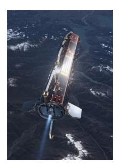
The sleek aerodynamic design of GOCE (Gravity Field and Steady-State Ocean Circulation Explorer) immediately sets it apart from most other satellites. This unique five-metre long spacecraft has none of the usual moving parts. The satellite together with its sensor, system of supporting instrumentation and control elements actually form a single composite gravity-measuring device. Credits: ESA - AOES Medialab
