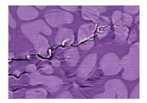
Cracks propagate through metallic glass by following shear bands, which in this micrograph look like wrinkles in cloth. The featureless blobs in the picture are a second, crystalline phase of the metal, but if these barriers are not properly spaced to halt crack propagation, the metal can fail disastrously. Credit: William Johnson, Caltech; Robert Ritchie, Berkeley Lab
