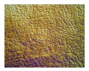
The two-phase structure of DH3, a metallic glass alloy of five different metals. When the space between the dendritic branches are properly spaced, they can stop cracks before they propagate. Credit: William Johnson, Caltech; Robert Ritchie, Berkeley Lab
