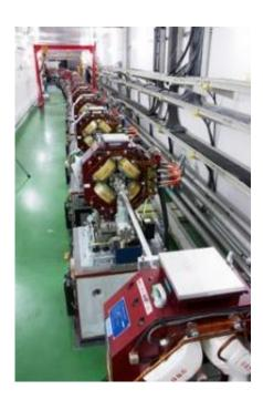
The Accelerator Test Facility 2 in Japan uses a 50-meter series of magnets to focus its electron beam. (Photo by N. Toge, KEK.)
