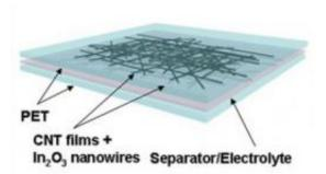
Anatomy of a supercapacitor: two films combining Indium Oxide  $(In_2O_3)$  separated by a layer of Nafion film. Credit: USC Viterbi School of Engineering
