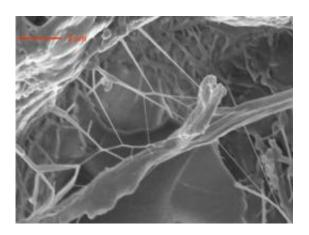
Researchers at Rensselaer Polytechnic Institute have discovered a new technique for provoking unusual crazing behavior in epoxy composites. The crazing, which causes the composite to deform into a network of nanoscale pillar-like fibers that bridge together both sides of a crack and slow its growth, could lead to tougher, more durable components for aircraft and automobiles. Credit: Rensselaer/Koratkar
