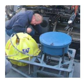
DEIMOS consists of an echosounder -- encased in a 17-inch diameter sphere of thick glass and then in a yellow plastic cover -- and a transducer set in a metal frame. Here Knut Brekke, a pilot of the remotely operated vehicle that will deploy DEIMOS, checks the set up. Credit: D. Kreisberg/University of Washington
