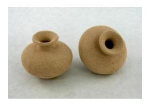
These pots were inspired by Southwest Native American pottery and created using potter's clay. They emerged from a high-tech 3-D printer before being fired in the usual way. The fine horizontal lines are an artifact of the printing process. Credit: University of Washington
