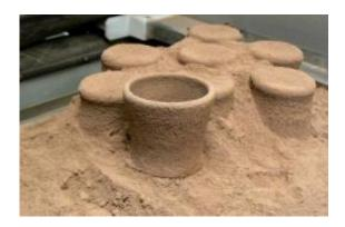
After printing, loose powder falls away from the printed ceramic objects. These cups were created using the UW recipe, which costs about 3 percent as much as commercial 3-D printing powders. Credit: University of Washington
