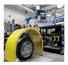
Argonne automotive engineer Henning Lohse-Busch puts an engine through its paces on Argonne's Modular Automotive Technology Testbed (MATT), a platform that allows different engine components to be observed and evaluated as they operate in a complete vehicular system.
