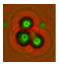
An experimental "cold fusion" device produced this pattern of "triple tracks" (shown at right), which scientists say is caused by high-energy nuclear particles resulting from a nuclear reaction Credit: Pam Boss, Space and Naval Warfare Systems Center (SPAWAR)
