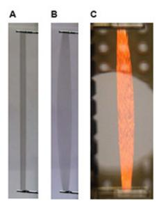
A. An artificial muscle strip with no voltage applied. B. The above artificial muscle strip with 5 kV applied. C. An artificial muscle strip actuated at 1500 K using 5 kV applied voltage.
