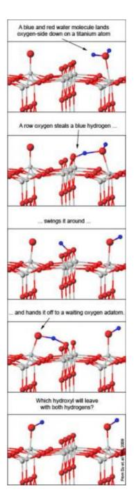
With the help of a single oxygen atom, the titanium oxide surface helps a water molecule split into two oxygen-hydrogen pairs called hydroxyls. Credit: Lyubinetsky/PNNL
