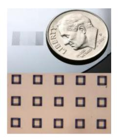
In the upper image, an array of mirored pyramidal wells is shown next to a dime. Each of the tiny dots in the array is a well shaped like an inverted pyramid, technically a truncated pyramid, one with its top cut off. Individual pyramidal wells are shown in the lower image. Each is about the width of a human hair. Image: John Russell/VIIBRE
